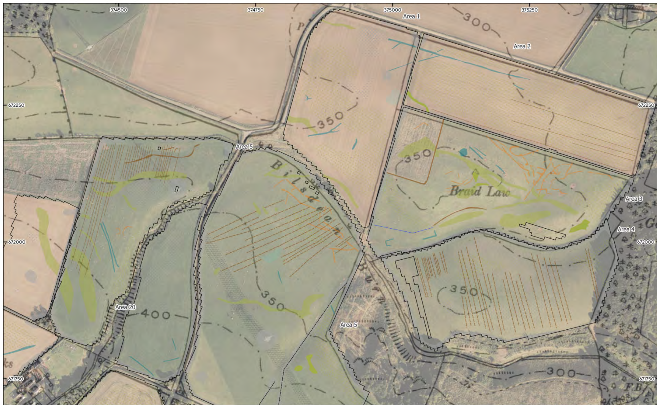
MSNT1875 - Springfield, East Lothian Figure 4 - Magnetic Interpretation over Historical Mapping & Satellite Imagery (Areas 1 - 5, & 20) 1:3,000 @ A3 © Magnitude Surveys 2025 Contains Ordnance Survey data © Crown Copyright and database right 2025
