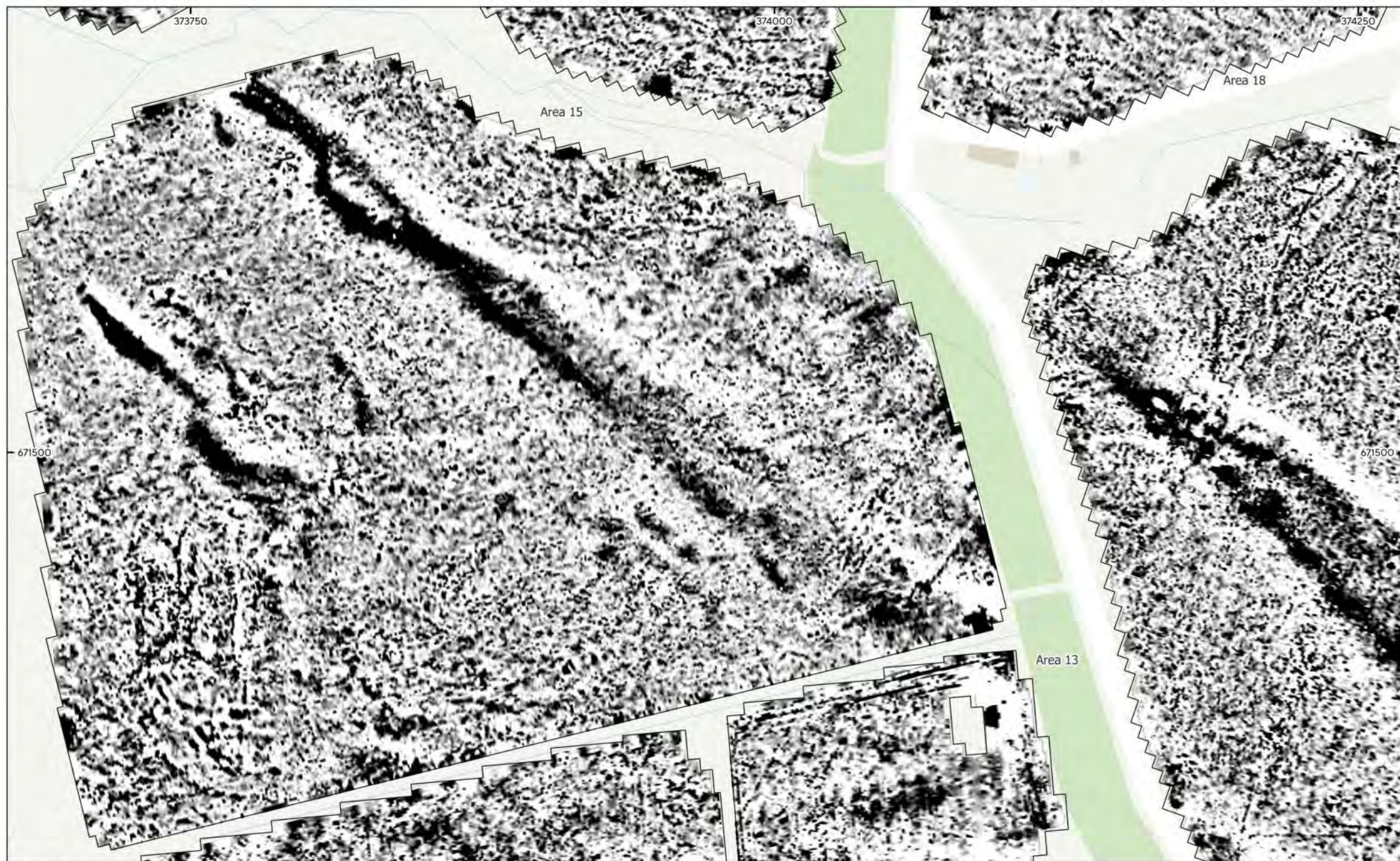
MSNT1875 - Springfield, East Lothian Figure 36 - Magnetic Gradient (Areas 13 & 15) 1:1,500 @ A3 © Magnitude Surveys 2025 Contains Ordnance Survey data © Crown Copyright and database right 2025
