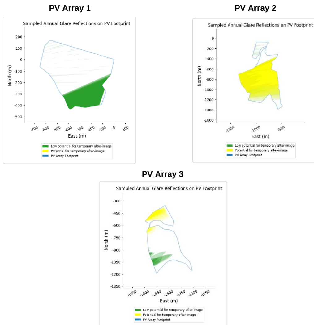
Figure 5-8: Area of PV Arrays where the glare emanates from
